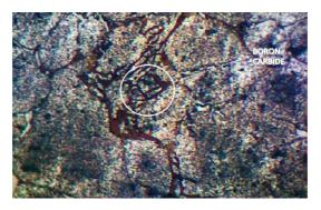
Fig: 6- Microscopic image of Al-B4C-Graphite (100 x)
