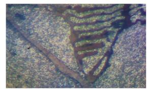
Fig: 7 - Microscopic image of Al-B4C-Graphite (400 x)
