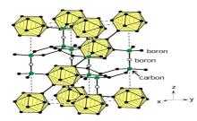
Fig 1 – Structure of Boron Carbide
