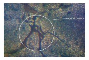
Fig: 6 - Microscopic image of Al-B4C-Graphite (200 x)
